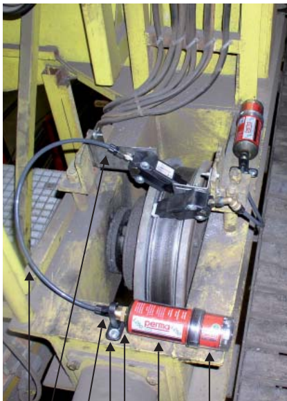
Nylon tube Tube Connection G1/4a Tube Connection f. perma G1/4i Bracket (stainless steel) STAR Support Flange G1/4a x G1/4i LC unit STAR VARIO drive
