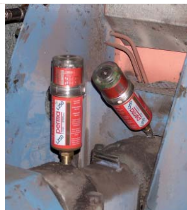
Lubrication system: 2 x perma STAR VARIO 250 cm 3
