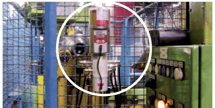
Permanent lubrication of various bearings and gear racks in the automotive industry. perma PRO guarantees safe, clean and efficient lubrication without the need to stop the equipment.
