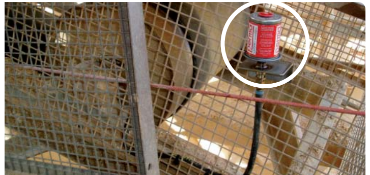
The remote installation of perma CLASSIC lubricator to this conveyor pulley bearing at a quarry has eliminated the need for safety cages to be lifted off for the purpose of lubrication. This reduces the chance of back strains associated with lifting safety cages and allows the lubricator to be inspected and serviced while the conveyor is operating.
