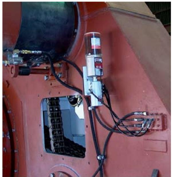
High-tech automatic lubrication for Drawworks.
