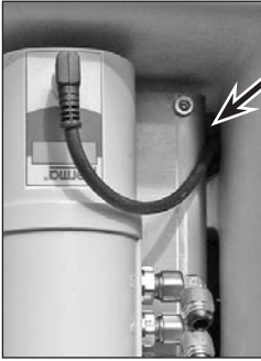
Fig. 10-1: Oblong hole for impulse and control cable in upper right hand corner of pump area
