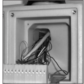
Fig. 10-1A: Square hole for cables in upper left hand corner of display area (picture shows additional cables).
