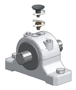
4. Lubrication point, accessory parts and tubes / hoses must be pre-filled with lubricant. This enables the lubricant to immediately reach the lubrication point.
