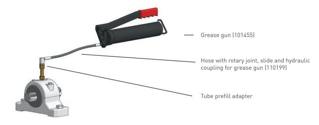
5. Prefill lubrication point and all grease lines for remote installation.
