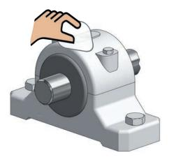
2. Remove grease nipple or plug screw of connecting thread and check thread size.
