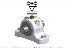
Pressure check: Lube-point / all connecting parts (refer to perma NOVA installation guide for details)
