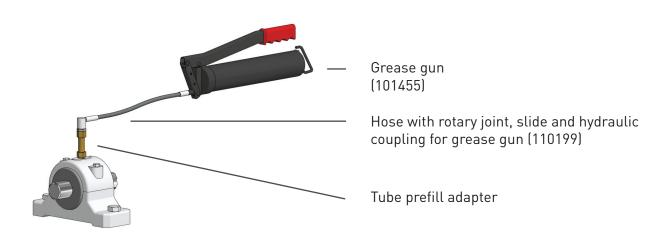
5. Prefill lubrication point and all grease lines for remote installation.
