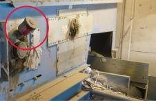
Lubrication of flange bearing on a conveyor
