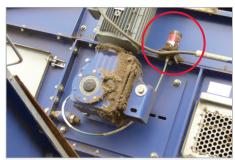
Lubrication of flange bearing on a conveyor
